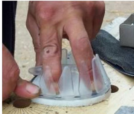
Fit cuff to base plate, you may have to cut tabs off of the cuff if foot is small. Stick cuff to base plate with superglue e.g. “Locktite 406”, press down until stuck.
